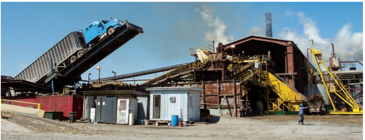
The bagasse remaining at the end of processing fuels the mill's boilers.
