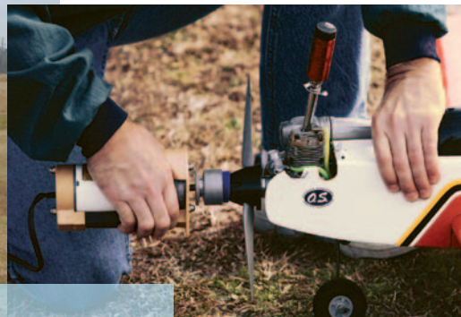
(Above) James Roteff attaches an electric starter to fire up his aircraft's fuel-powered engine.
