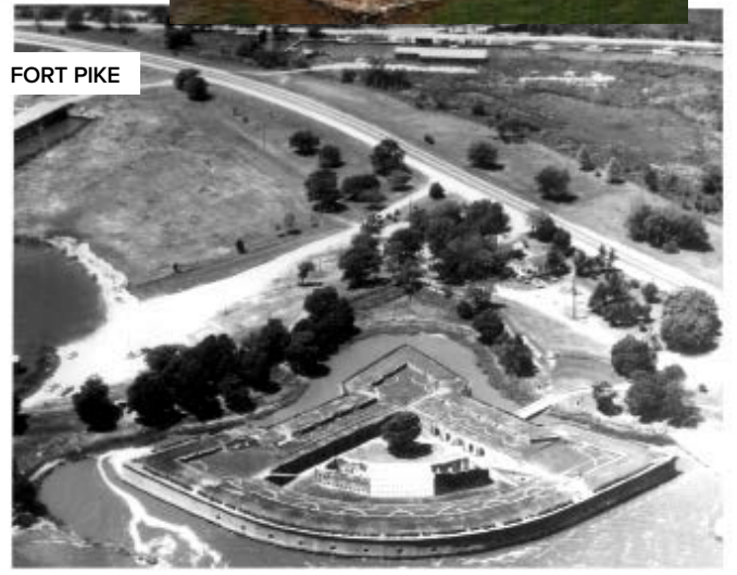
This 1972 aerial view shot by H.C. Willem Jr. shows the fort, inner court with citadel, gun emplacements, hot shot furnaces, moat and surrounding area of Fort Pike.
